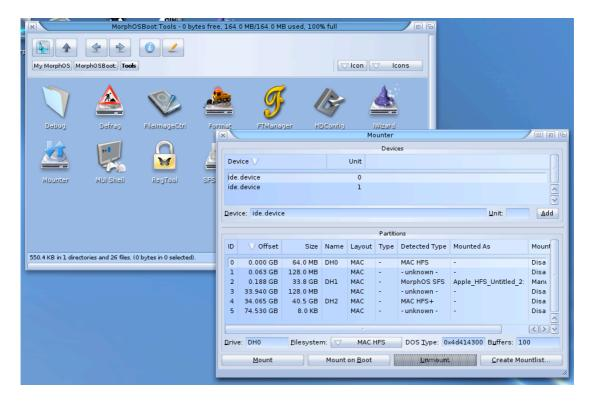
If the DH1 partition has '-' in the Mounted As column, select it and hit Mount (Filesystem must be either Autodetect or MorphOS SFS).
