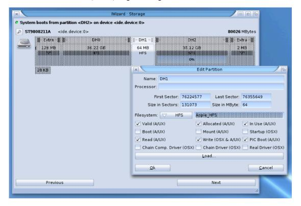
Last will be the partition for the MorphOS installation. Name it DH2 and make sure the Boot (A/UX) and Mount (A/UX) flags are turned ON. Change the Filesystem to SFS.
