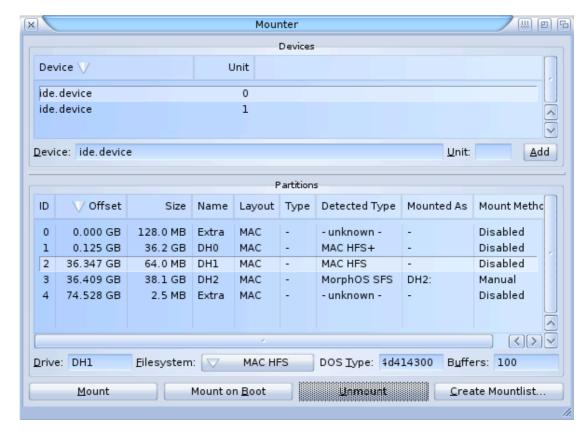
If the DH2 partition has '-' in the Mounted As column, select it and hit Mount (Filesystem must be either Autodetect or MorphOS SFS).
