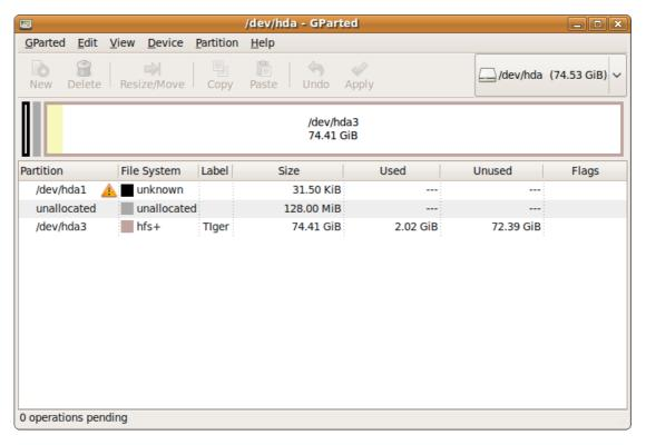
Select the OSX hfs+ partition and click on Resize/Move. Resize the partition by clicking and dragging on its right edge. Do NOT move the partition from its left edge. You MUST disable the Round to cylinders checkbox, or GParted will try to move the OSX partition. Make sure the Free Space Preceding (MiB) field stays at 128. You should leave at least 1GB of free space following the OSX partition. I'd recommend around 20GB. Now click on the Resize/Move button to apply your changes.
