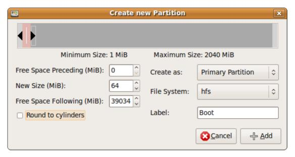
Select the unallocated space again, change the File System to unformatted (we will change it from MorphOS later), disable the Round to cylinders checkbox and press Add.
